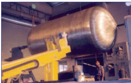
Filament wound composite pressure vessel.
