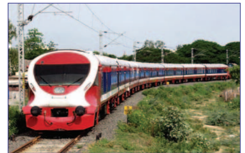
The front-end of this diesel locomotive for hauling passenger trains of Indian Railways was made by the vacuum infusion process.
